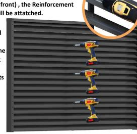
Here at this stage in cases when the Fence is longer than 2400mm The Reinforcement Profile will be higher than the Fence and will have to be adjusted with GREAT attention to be supported in the lower concrete base!!!
