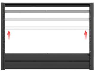
In step four we start the installation of the slats, the first upper slat will be installed and fixed first with rivets in front and then behind the fence (together with the Top Profile). The next slats one after the other will be fixed only from the front.
